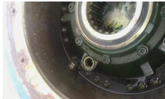
Figs. 3 and 4: Interior of winch drum showing ordinarily inaccessible planetary gear and filling plugs that have fallen out. Note that there was no external indication of an oil leak.
