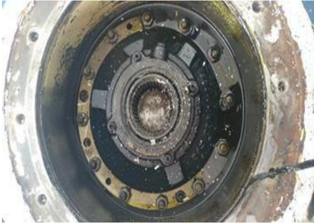
Figs. 5 and 6: Interior of above reduction gears after running in a dry condition leading to overspeed damage
