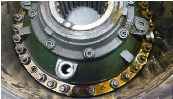
Figs. 3 and 4: Interior of winch drum showing ordinarily inaccessible planetary gear and filling plugs that have fallen out. Note that there was no external indication of an oil leak.
