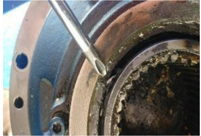
Figs. 5 and 6: Interior of above reduction gears after running in a dry condition leading to overspeed damage
